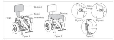
Take A6T from the packing container. Align the screws on backrest hinge to the screw holes and body holes, tighten screws (see Figure 1) and stick saddle to frame(see Figure 2). Pull outward and rotate the index plunger (see Figure 3) and get the mount stuck and loosen the index plunger (see Figure 4); rotate the armrests to horizontal position(see Figure 5 - arrow). Pull outward and rotate the index plunger and release it when a click sound is heard.
