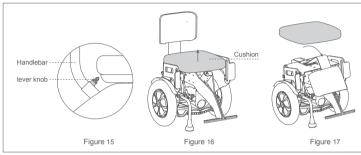
Rotate the lever knob. After hearing a "click", pull out the handlebar (see Figure 16), tear up the cushion tape (see Figure 16), remove the cushion. Then rotate the backrest in the direction follow the arrow in Figure 17, fold the backrest, and then attach the cushion to the body to complete the folding.
