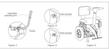
♠ Loosen the set setscrew (see Figure 11) to remove the adjustable operating arm from the body. Pull outward and rotate the index plunger (see Figure 12) and get the mount stuck and loosen the index plunger (see Figure 13); rotate the armrests to horizontal position (see Figure 14-arrow). Pull outward and rotate the index plunger and release it when a click sound is heard. Then the armrest is folded
